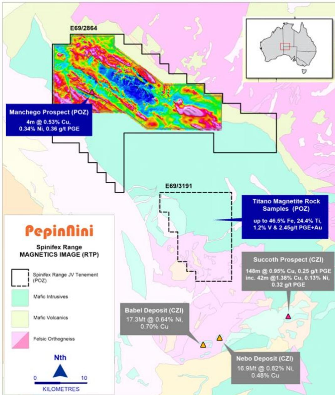
**Figure 1:** Spinifex Range (E69/2864) high-resolution airborne magnetics image (RTP) overlying regional geology and Ni-Sulphide occurrences
