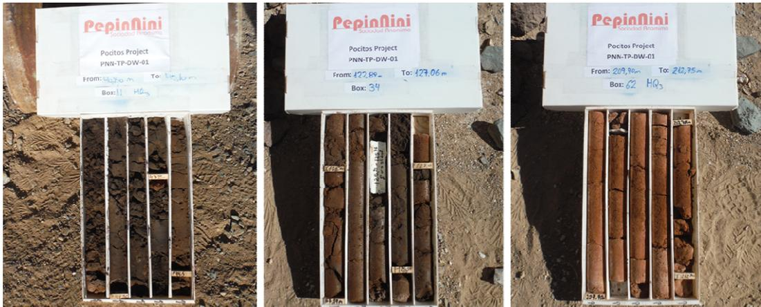
Figure 5 - Core samples from three main lithology intervals
