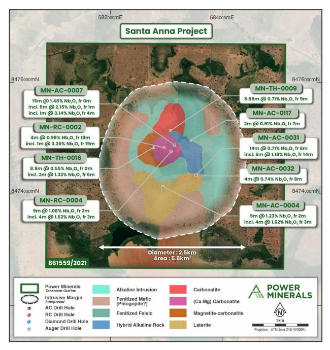
Figure 2. Santa Anna Project plan showing previous drillhole locations and significant niobium drilling results.
