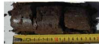
Photo 7: Core samples for Porosity testing
