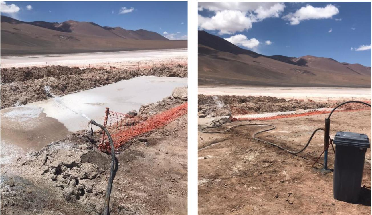
**Figure 1:** Airlift test of lithium brine flow rate, drill hole PM22-IN-002, Incahuasi salar
