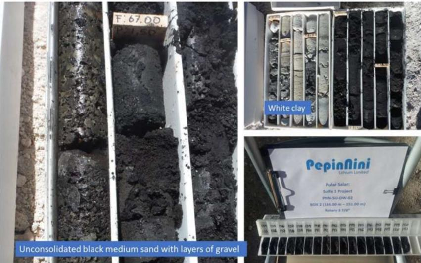
DRE B BOXES SHOWING ALL THE LITHOLOGIES AFOREMENTIONED, AT A DIFFERENT DEPTH, CUTTING BOX LOG,
