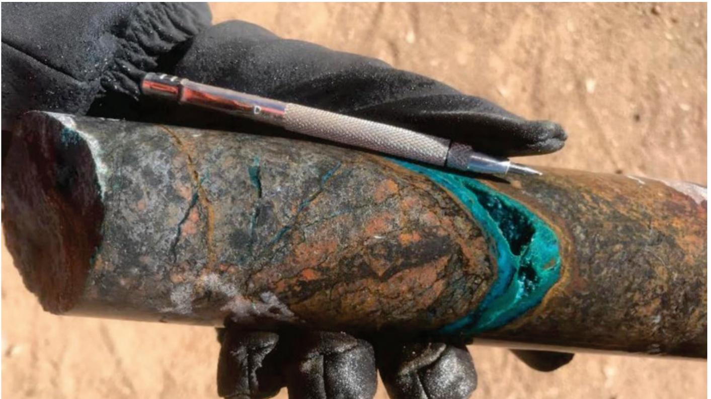
Figure 11: Drill core from hole PNSI22-001 at 89m showing quartz-malachite-azurite-chrysocolla veins
