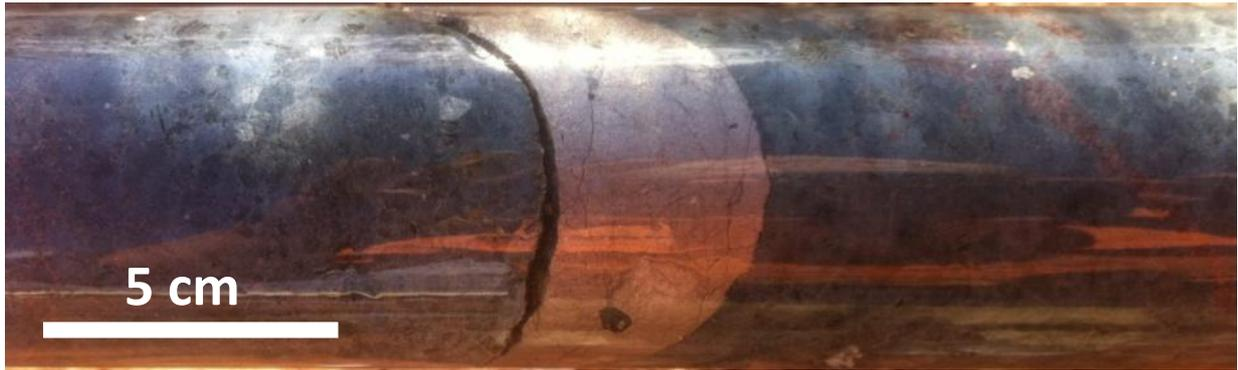
**Figure 1:** DD12COP015, Vein of massive pyrrhotite cross-cutting the fabric of a felsic gneiss (162.5m depth)
