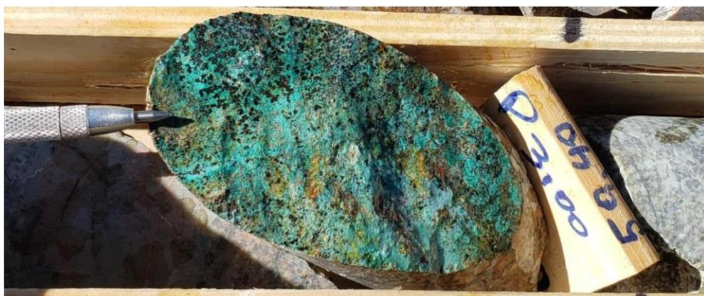
**Figure 7:** Drill core from hole PNSI22-002 at 59.4m showing quartz-biotite-magnetite veins with Cu-Fe oxides
