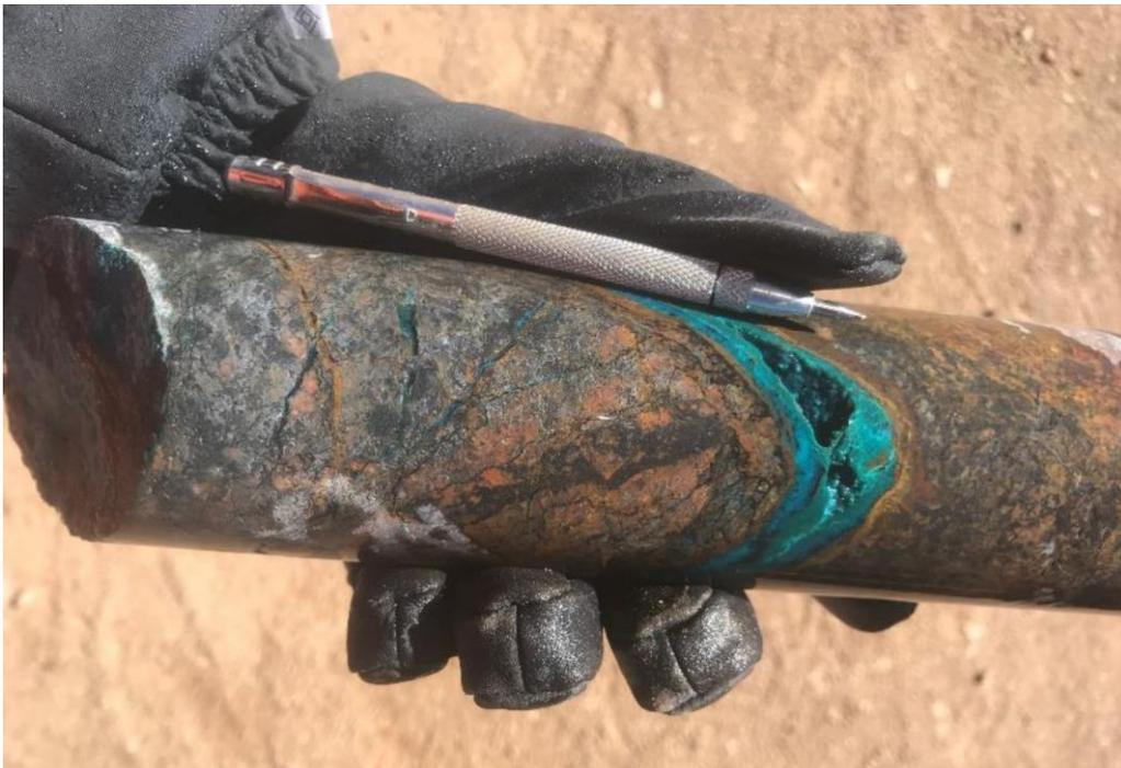
**Figure 6:** Drill core from hole PNSI22-001 at 89m showing quartz-malachite-azurite-chrysocolla veins
