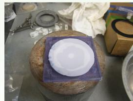
Figure 2. Test cell assembly with micropore filter paper at bottom
