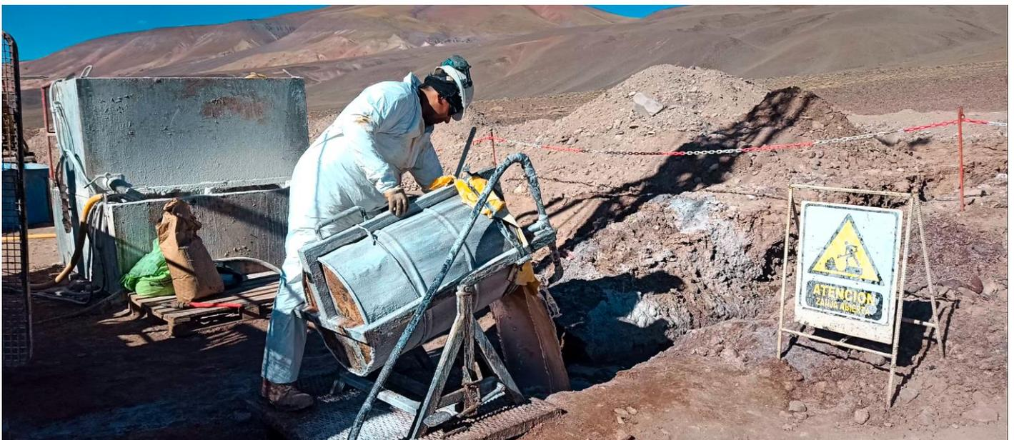
**Figure 1:** Brines packer testing at drillhole PM23-IN-04 at Incahuasi salar, Salta Lithium Project.
