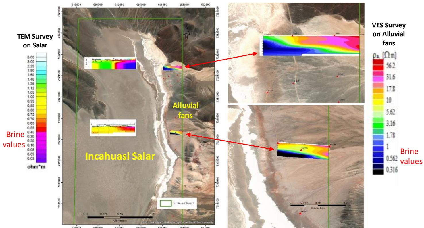
**Figure 3:** Comparison of previous TEM geophysical survey (left side = active salar) with recent VES geophysical survey (right side = eastern alluvial fan apron), Incahuasi salar.
