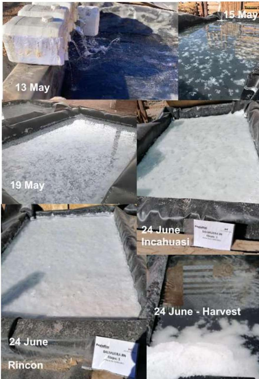
Figure 6 Brine Evaporation Concentration Sequence
