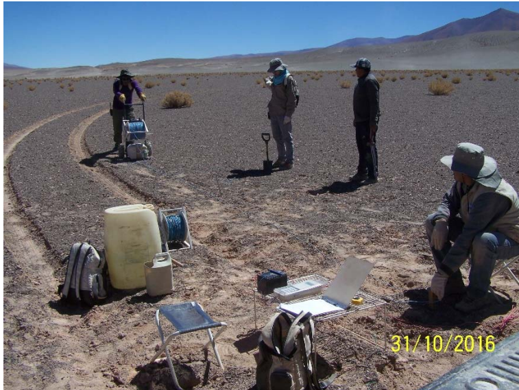
Figure 4 – VES survey Salar Pocitos, Salta, Argentina
